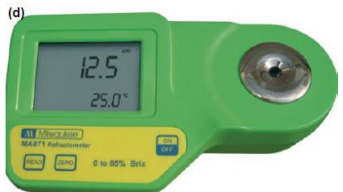
Figure 3: Digital refractometer used to measure °Brix levels in control and treated grapes.
