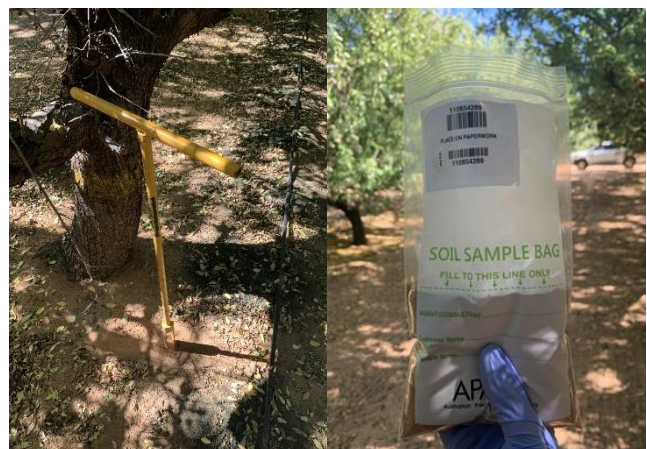
Figure 1: Images of soil sampling for the Re-Leaf® trial. Soil samples were taken 30cm deep and sent to APAL for analysis.
