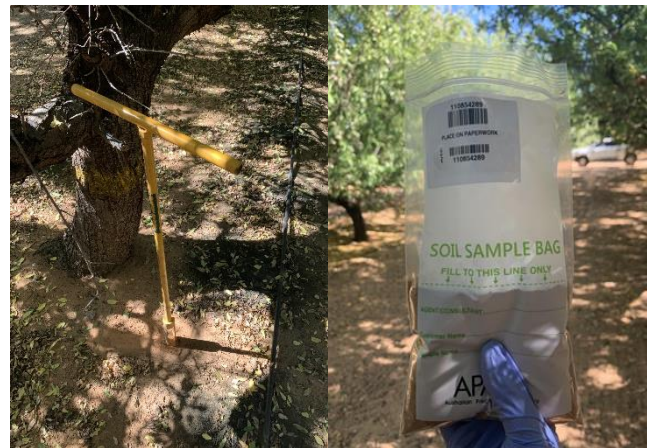
Figure 1: Images of soil sampling for Complete Blend 10® trial. Soil samples were taken 30cm deep and sent to APAL for analysis.
