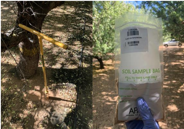
Figure 2: Image of soil sampling for Complete Blend 10 ® trial. Soil samples were taken 30cm deep and sent to APAL for analysis.
